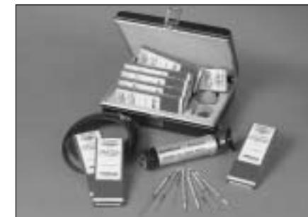
Model 8014KA Toxic Gas Detector Tube System
